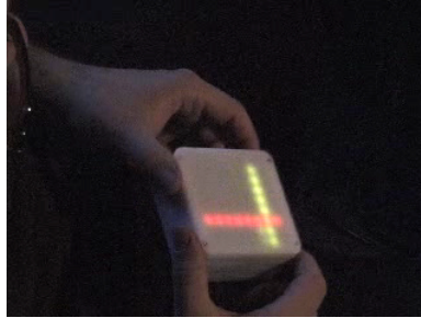
Figure 3.11: Levin and Yarin's. prototype of the acceleration-based interface. The lines move along the x and y axis when the device is tilted. From "Bringing sketching tools to keychain computers with an acceleration-based interface ( Levin and Yarin, 1999 ).
