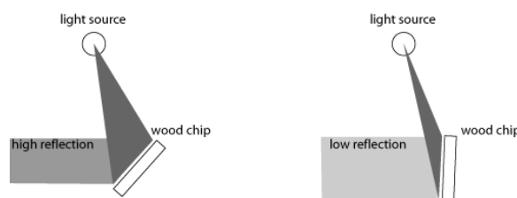
Figure 4.16: Principle of reflecting light from tilted wood chips.
