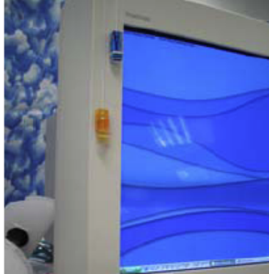
Figure 3.16: Ambient Beads. Each bead is suspended by a thin wire from the top of the monitor, and a small motor controls the height of the bead by reeling the line in or out. A continuous motion, or motion at regular-intervals, may be mapped to an approaching event in time. The changed position of a bead could be mapped to a friend's online status: "up" or "down." Image ( Elliot and Greenberg, 2004 ).
