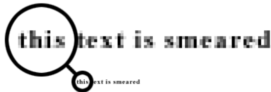
Figure 4.2: Text smeared by anti-aliasing.
